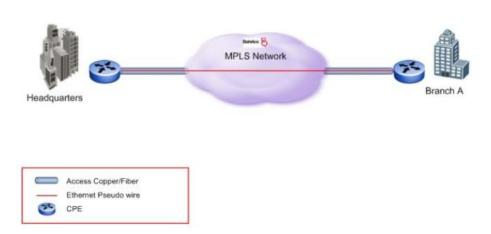
B. Layer 2 Hub & Spoke (Point-to-Multipoint) is provided over Layer 2 with traffic routing under full control of the customer. It is ideal for companies that require connectivity between their headquarter and branches. All the virtual circuits terminating from the spoke sites are aggregated on a single physical link at the hub site.
