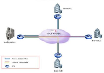
C. Layer 3 IP-VPN Full Mesh (Multipoint-to-Multipoint) offers any-to-any connectivity between multiple locations with traffic routing managed by Batelco's VPN network. It is ideal for
